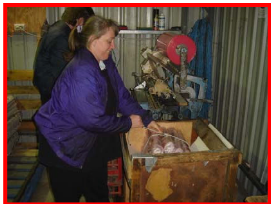
Figure 34: Wooden base in container reduces lumbar spine flexion.
